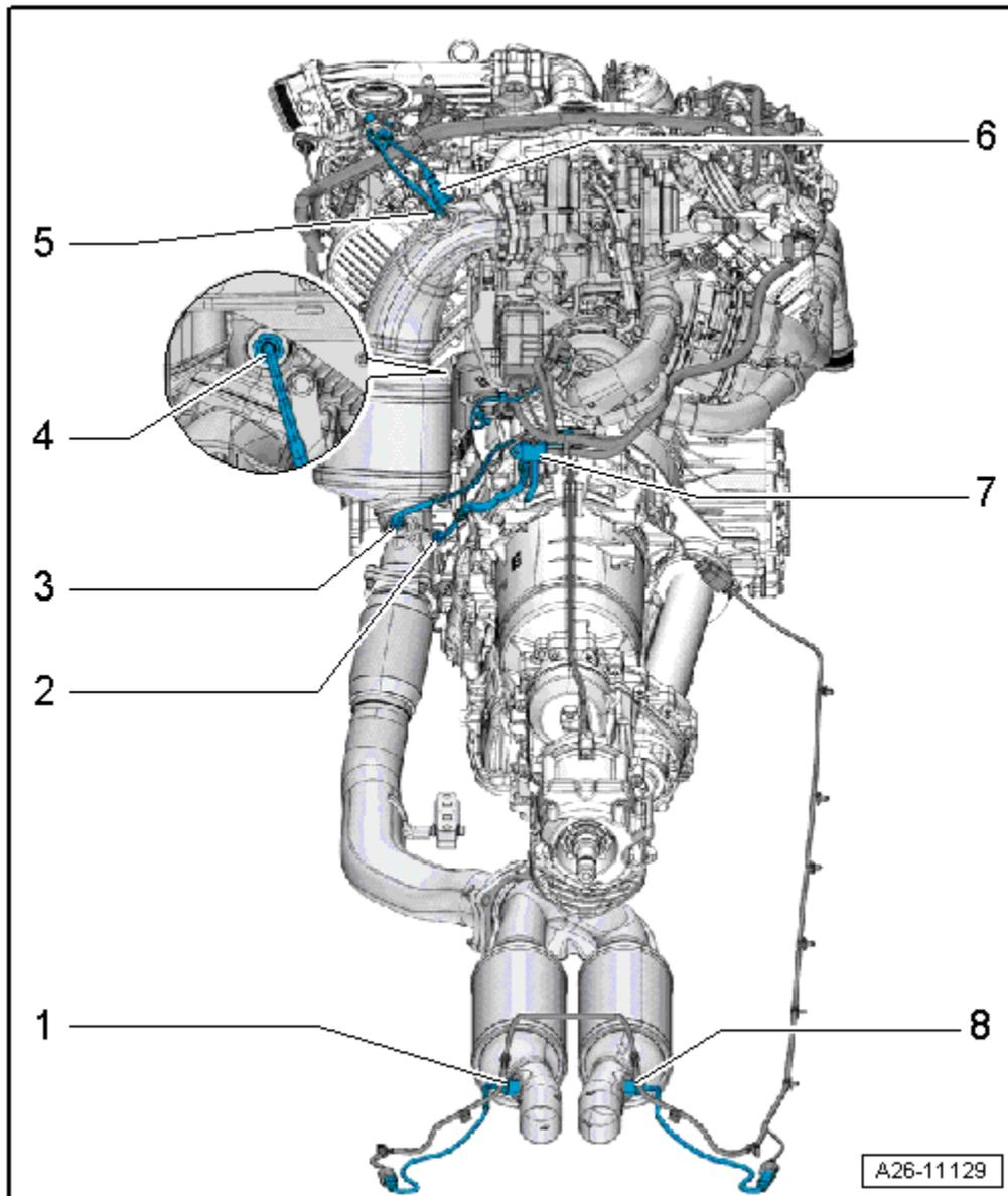
1 - Exhaust gas temperature sender 4 for cylinder bank 2 -G649-
